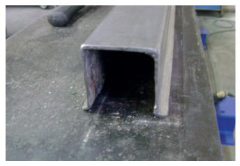
Afterwards: Stopend formwork as good as new: Straightened stopend formwork with optimised function
