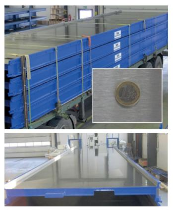
After renovation: closed, polished and straightened formwork surface is as good as new; paintwork completely overhauled and as good as new
