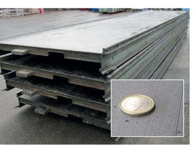
Poor quality of a pallet formwork surface before renovation: deep scoring and uneven formwork surface; poor paintwork
