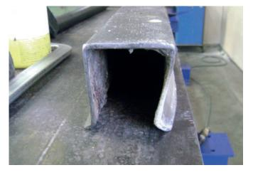
Before renovation of the stopend formwork systems: Deformed and dented stopend formwork
